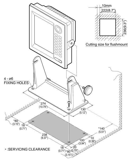
Figure 5-11 How to mount the display unit
